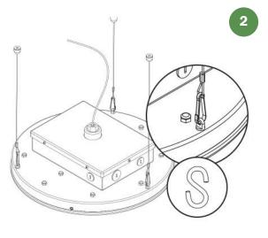
Recommended: Zinc Plated S-Hook and Galvanized Steel Cable
