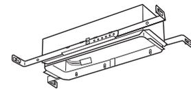
2. To install the LED Strip, remove the protective film on the double sided VHB tape and place in the selected location. The LED strip must be centered in the mounting area of fixture. Once it is set, apply pressure to ensure a proper bond with the VHB tape and the fixture. If there are any parts of the housing blocking a secure connection with the VHB tape, use extra VHB tape and layer it until it provides a higher mounting point for the kit.
